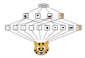
**FIGURE 10.6.** Schematic showing how a convolutional neural network classifies an image of a tiger. The network takes in the image and identifies local features. It then combines the local features in order to create compound features, which in this example include eyes and ears. These compound features are used to output the label "tiger".
