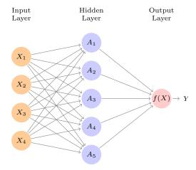
FIGURE 10.1. Neural network with a single hidden layer. The hidden layer computes activations  $A_k = h_k(X)$  that are nonlinear transformations of linear combinations of the inputs  $X_1, X_2, \ldots, X_p$ . Hence these  $A_k$  are not directly observed. The functions  $h_k(\cdot)$  are not fixed in advance, but are learned during the training of the network. The output layer is a linear model that uses these activations  $A_k$  as inputs, resulting in a function f(X).
