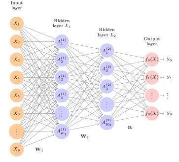
**FIGURE 10.4.** Neural network diagram with two hidden layers and multiple outputs, suitable for the MNIST handwritten-digit problem. The input layer has p = 784 units, the two hidden layers  $K_1 = 256$  and  $K_2 = 128$  units respectively, and the output layer 10 units. Along with intercepts (referred to as biases in the deep-learning community) this network has 235,146 parameters (referred to as weights).
