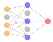
**FIGURE 10.19.** Dropout Learning. Left: a fully connected network. Right: network with dropout in the input and hidden layer. The nodes in grey are selected at random, and ignored in an instance of training.
